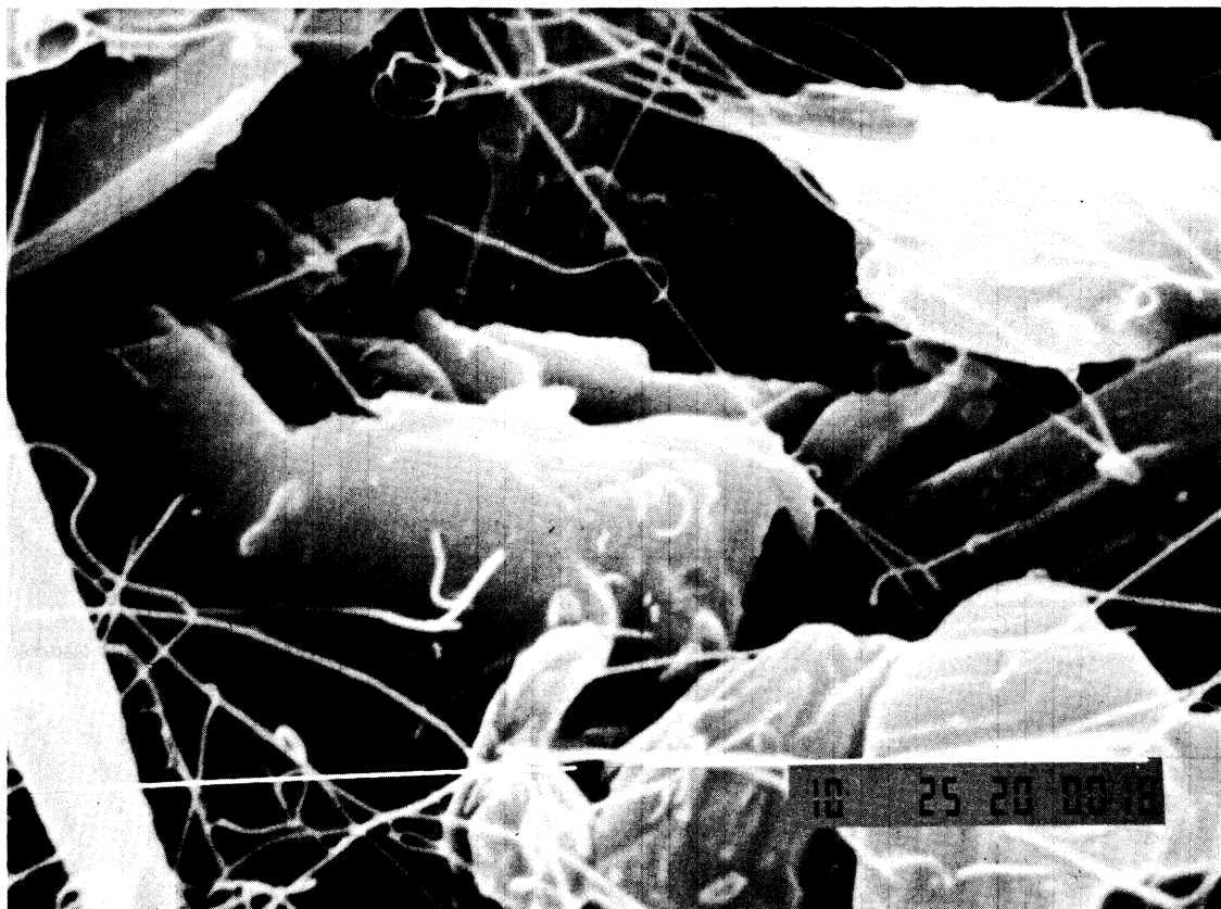
FIGURE 5. Scanning electron micrograph of the surface of a \text{TTF}^+\text{TCNQ}^- electrode. The strands of polymer binder can be seen.
